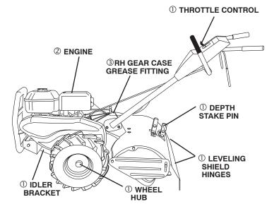
①SAE 30 OR 10W-30 MOTOR OIL ②REFER TO MAINTENANCE "ENGINE" SECTION ③EP #1 GREASE
